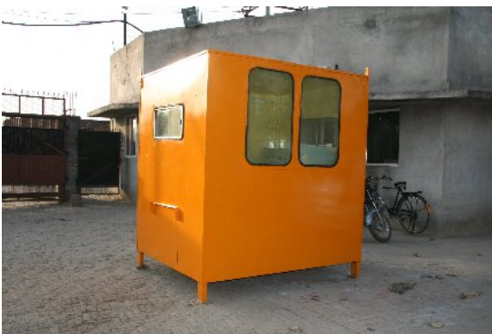
The plant is provided with a fully automatic batch control system located in a stand alone cabin which is spacious and clear view of the plant
