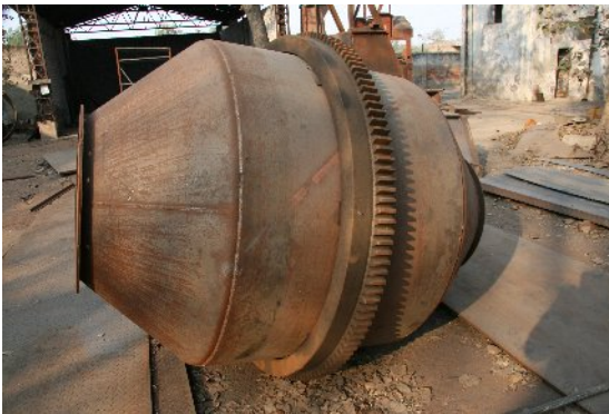
The reversible steel drum is fabricated of high manganese steel which has a long life the complete drum gear is fabricated in house on an imported hobbing machine.
