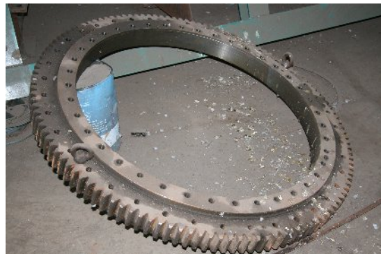
The slewing ring for the drum of the mixer is completely imported, hence giving the drum a long lasting life.
