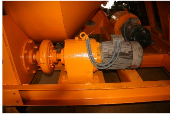
A 10 HP motor operates the drum during mixing and dumping of the concrete
