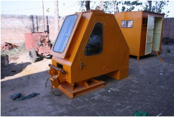
A view of the operators cabin for the Boom Scrapper which is mounted on a slewing ring
